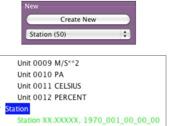
Our station will consist of three broadband channel components. Let's go ahead and add a single channel that we can replicate to the other two components. We will do a *Create New* action using the "*Channel (52)*" selection, making sure that we have the station still selected.
