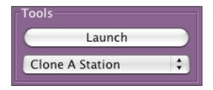
Select a station that represents the instrumentation you want to clone into new stations. In the *Tools* button group, select *Clone A Station*. When you hit *Launch*, you are presented with a tool for specifying any number of new station names, along with the typical data fields that are different from the original station.
