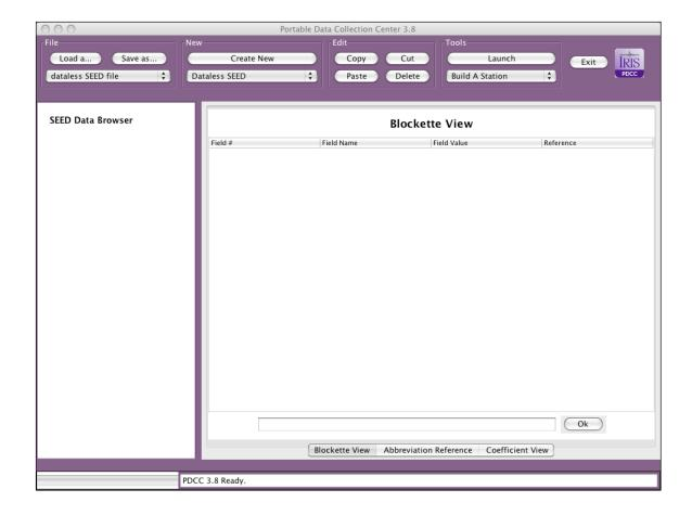
The opening view of PDCC shows you a toolbar along the top with groups of buttons, a SEED file browser window along the left hand side, and a blockette edit window with tabs along the right. On the bottom is a status bar.
