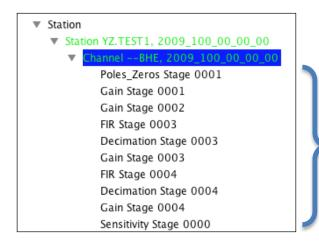
The blockettes are ordered from the first stage to the last stage of the instrumentation response. The very last response stage should always be '0', which is an overall *sensitivity* response. The *NRL Tool* supplies a computed value for the instrument sensitivity and places this value in the *sensitivity* blockette.
