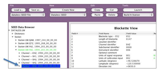
Upon selecting a channel, refer to the *Tools* button group. Make sure that the combo box is selected to *Select Instrumentation*. Then hit the *Launch* button.
