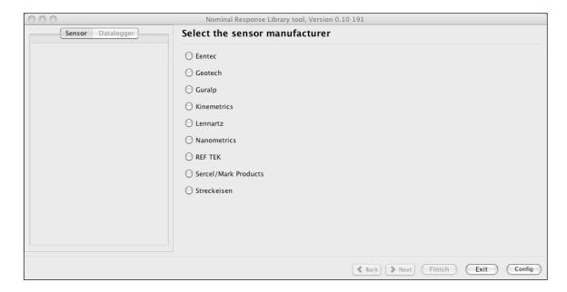
The first goal is to specify the *sensor type*. You start by indicating the manufacturer, then a model number, and then specify additional parameters. This tool operates like a wizard, where you make an entry and then select *Next* to continue.
