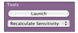
This is a simple feature to run a recalculation of the current response stack in a selected channel in your dataless, the output of which is the sensitivity of the channel. This value gets inserted into the Blockette 58, Stage 0 of your channel's response stack automatically, the same way as NRL Tool does.
