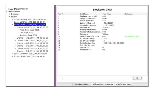
The table is a representation of the contents of that blockette. Each row is a *field* in the blockette, complete with the field name, the value, and any special *references* that may come from that field (abbreviations and coefficients).
