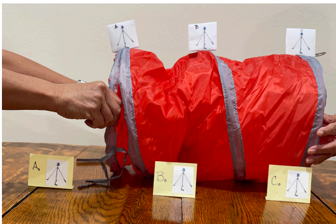
FIGURE 8. Uncompressed (top) and compressed (bottom) spring tunnel. Notice that the spring is pushed halfway between the first 2 GPS images on the ground. The first 2 GPS stations on top have moved, with the GPS A, closest to the force (on the left), moving the most. The image at position C shows no movement from the original position shown on the ground below. This depicts the compression of the North America plate due to the subducting Juan de Fuca plate.
