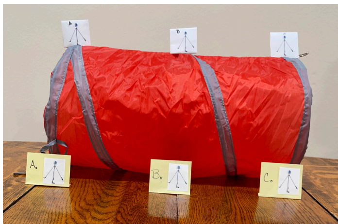
FIGURE 7. ORIGINAL GPS POSITION MARKERS. Attach the sticky notes with GPS stations on the ground or table, aligned with the stations on the spring.
